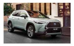
A hybrid uses both petrol and electric motors to provide power to the wheels. There is a battery to power the electric motor which is charged by the petrol engine when not being used. The engine management system decides when to use the electric motor (normally at low speeds or when accelerating) and when to use the petrol motor.
